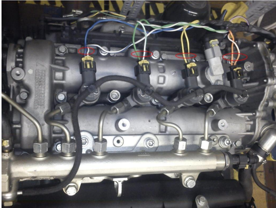
Fig. 1. Fiat 1,3 tdi common rail engine and voltage supply wires for injectors
